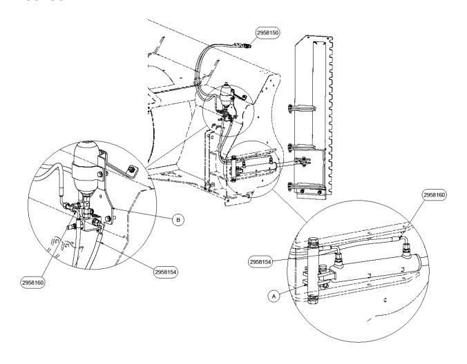
A: The bracket for the cylinder must be installed as in the illustration. B: 2 pcs. holes threaded M10.
